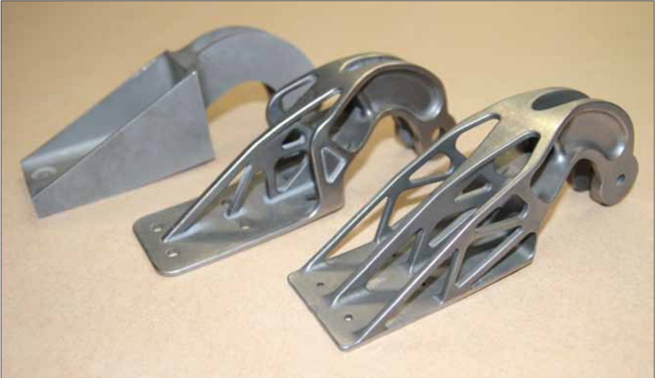
Traditionally manufactured hinge, prototype hinge and final printed hinge
