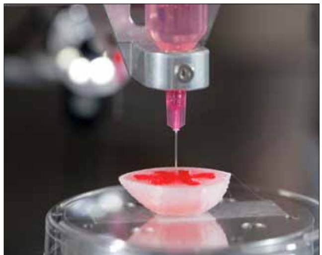
3D printing with 'ink' containing cells
